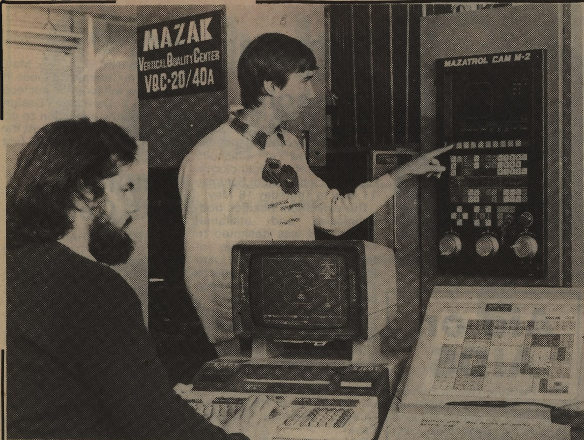
Fourth year engineering students, John Simmons (at keyboard) and Bruce Olsson, demonstrate the direct CAD-CAM link.
