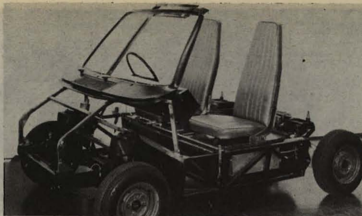
ABOVE: A close-up of the basic structure of the Flinders electric car. BELOW: The car undergoing a test run near the university.
