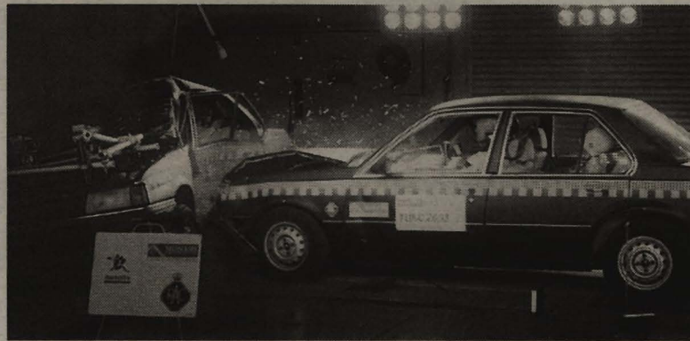
A test-dummy 'driver' in the vehicle at left is used to test the new seat-belt pre-tensioner under side-impact conditions.
