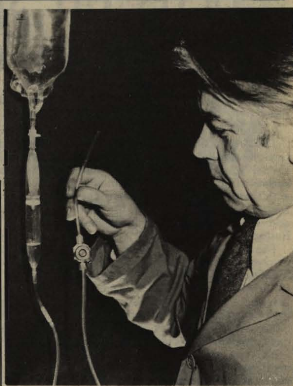
Senior technical officer, John Macleod , with an intravenous drip control prototype using his 'rolling diaphragm' valve invention. At top, a close-up. Photos: Peter Herforth .
