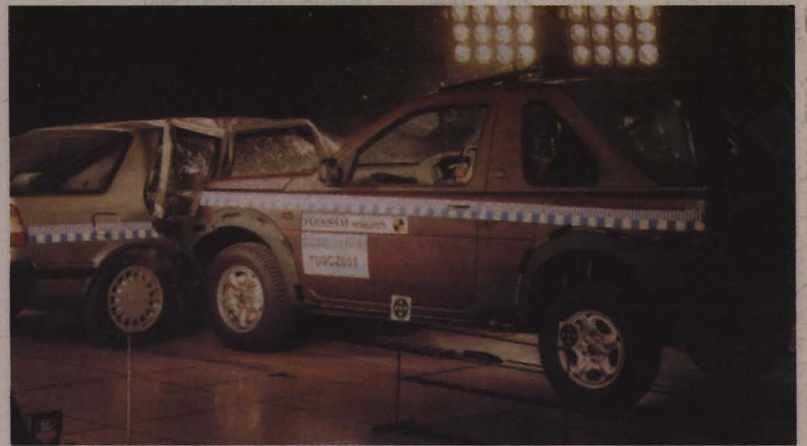
Unfair advantage: A four-wheel drive causes much more damage to a car in a side-impact crash than another car would, according to MUARC test results.
