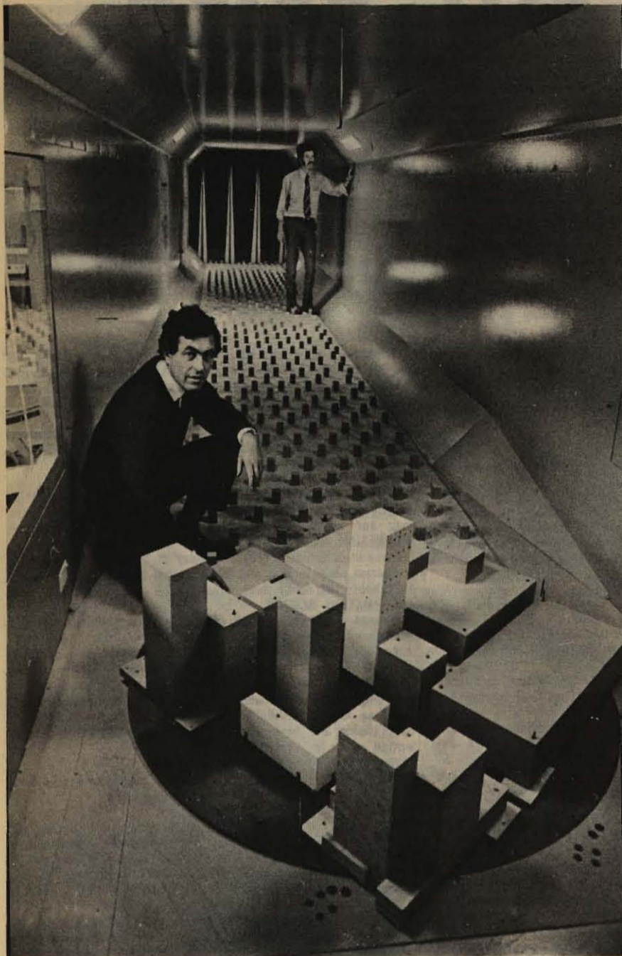
ABOVE: The wind tunnel in Mechanical Engineering, showing Dr. W. H. Melbourne at a model of a set of Melbourne city buildings. The model is on a turntable that can be set in any direction to the wind.
