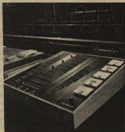
THE student response system in operation at Melbourne University is pictured above. Below is a close up of the lecturer's console with the arrangement of lights. A low screen, absent here, normally shields the display from the student view.
