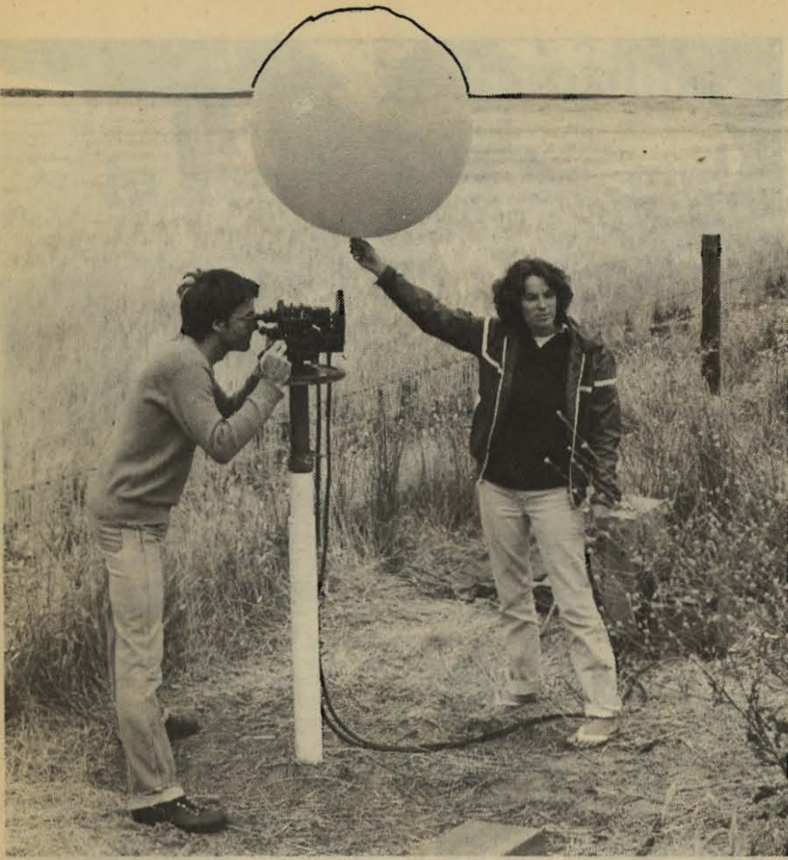
ABOVE: A CSIRO plane, with instruments in its nose, on standby for a cold front "alert". LEFT: Monash student Cathy Joyce releases a helium-filled balloon which is tracked by double theodolites.
