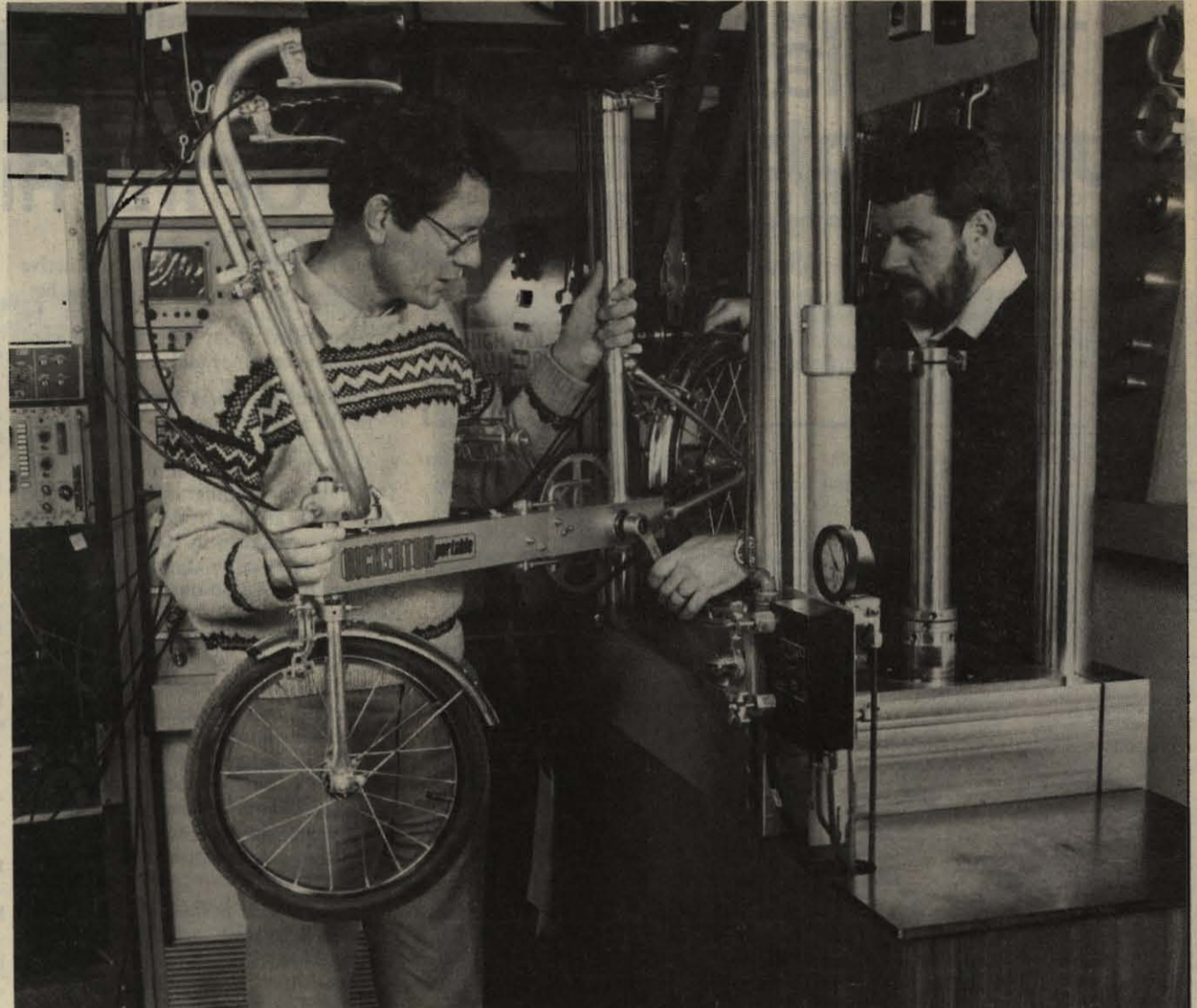
Dr John Griffiths, senior lecturer in Materials Engineering, and laboratory assistant, Mike Johnstone, test the bike for "fatigue". Open Day visitors will be able to see the department's fatigue machine in action. The test replicates a project undertaken for an Australian manufacturer to ensure the bicycle met the Japanese industrial standard for bicycles. With weights attached to the saddle post and pedals, it was heavily jolted through 70,000 cycles at 450 cycles per minute to test for distortion or cracks to the frame. Below: Former Monash Activities Officer, Graham Dean, who is currently deputy director of Open Day. Photo: Julie Fraser.
