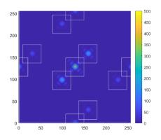
This image shows the two-dimensional FFT of a captured image with several information-carrying "channels" highlighted. The goal of the project is to shape the illumination to create maximum separation between these channels and design extraction filters using a single, end-to-end, artificial intelligence/machine learning system.
