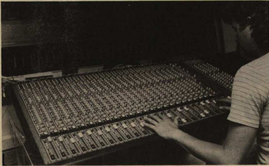
● Technician David Marmo operating the new Harrison MR4 28-channel audio-mixing console recently installed in Robert Blackwood Hall.
