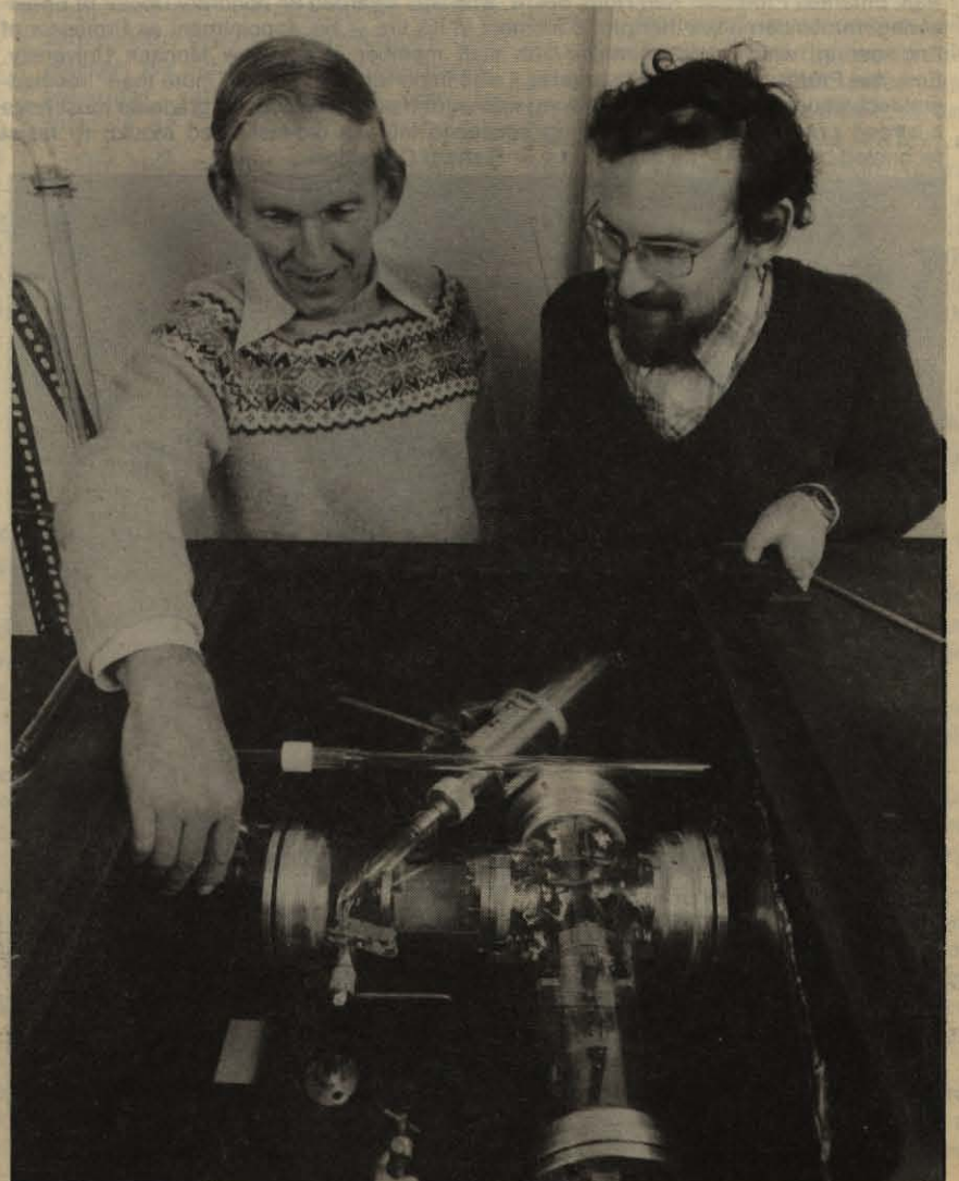
• Michael O'Dwyer, left, and Don McGilvery inspect the white-welsh multiple reflection fluorescence cell which will be on display in the Chemistry department.
