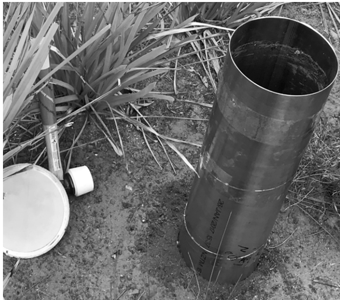
Figure 1. Revised Modified Philip-Dunne infiltrometer
