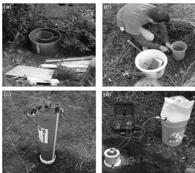
Figure 3. The methods of measuring infiltration rates in a biofilter (a) double-ring infiltrometer, (b) single-ring infiltrometer, (c) MPD infiltrometer, and (d) automated SATURO infiltrometer (Ebrahimian et al. 2020)
