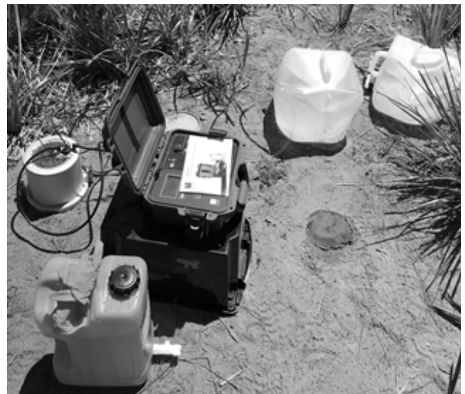
Figure 2. SATURO infiltrometer set up at a biofilter in Monash University, Clayton
