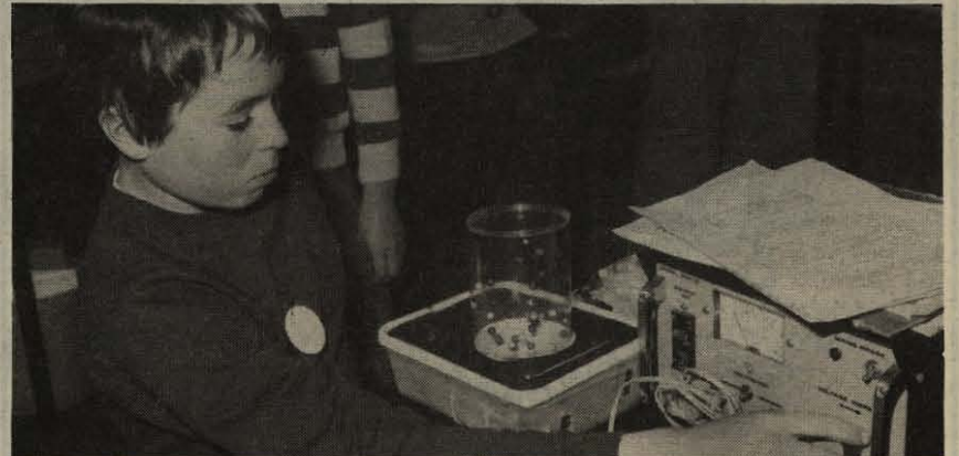
• Tony Robertson of Wheelers Hill High School with the equipment he designed and made to demonstrate the motion of molecules. A power pack is used to activate polystyrene balls representing molecules, to show how they react in solids, liquids and gases.
