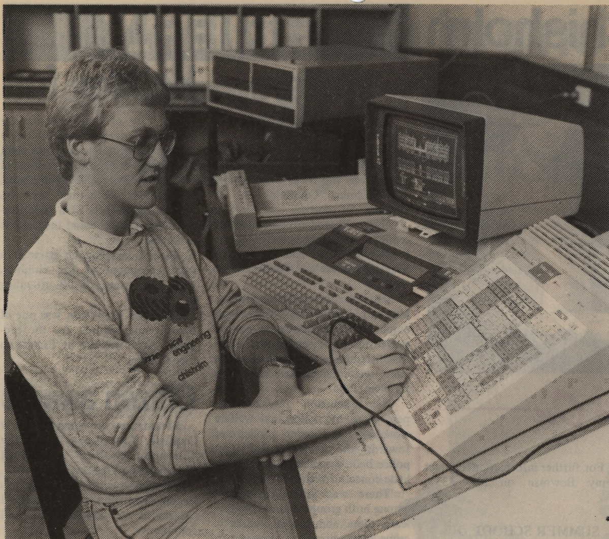
Final year Mechanical Engineering student, Stephen Jackson at the Controls of the Computer Aided Drafting (CAD) system which, when linked to the new MAZAK machine tool, will revolutionise the design and production process of engineering components.
